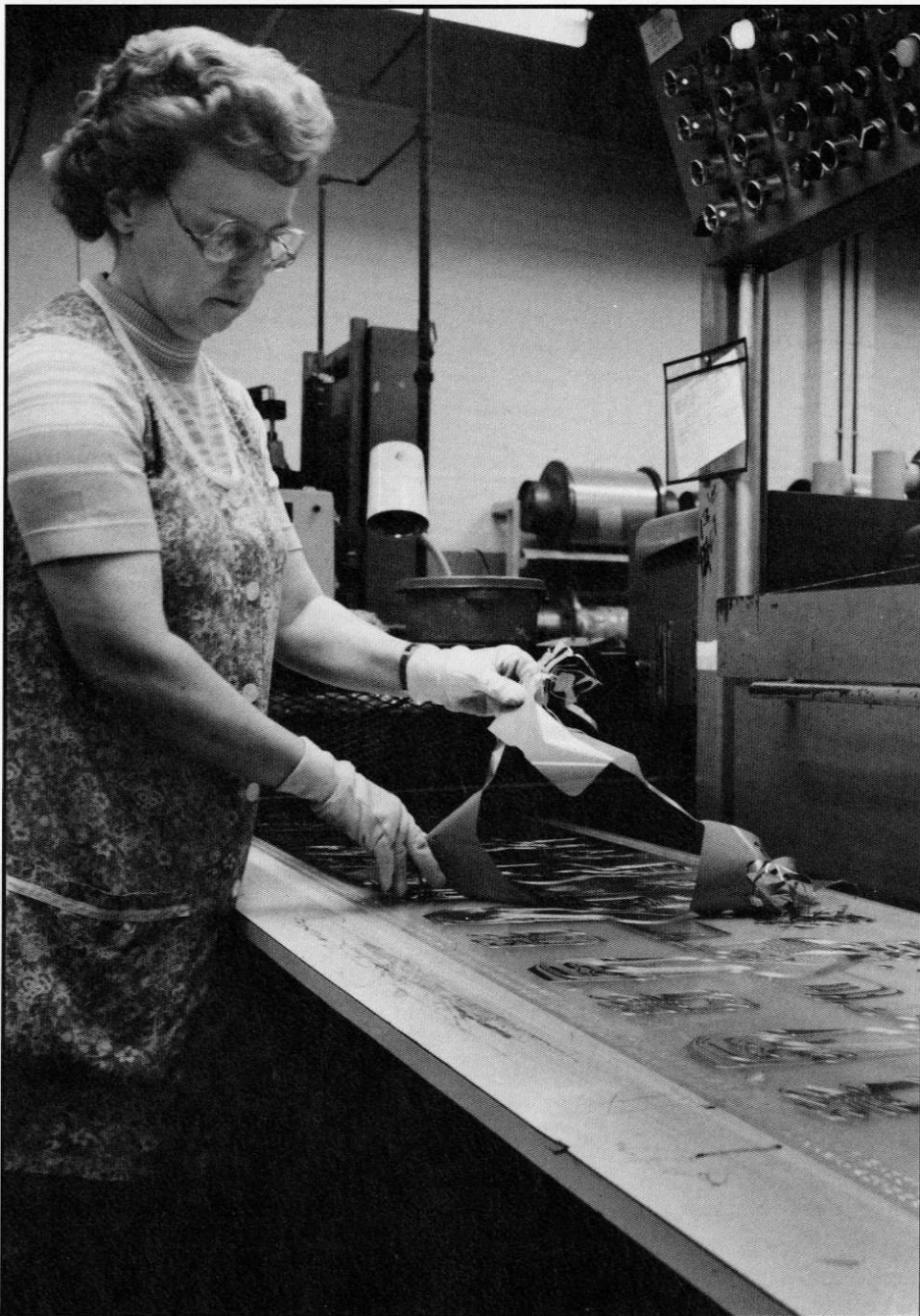
Wilma Heater, emboss operator, Dept. 334, strips excess copper from the mylar substrate.
