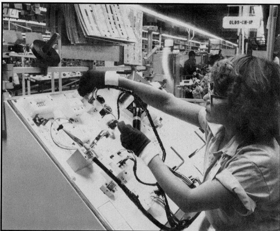
Mary Carmen Hernandez, utility operator, Cableados, uses the ALRO (At Line Ring Out) system to perform a full-function electronic test on a 1986 Oldsmobile C-H Instrument panel harness.
