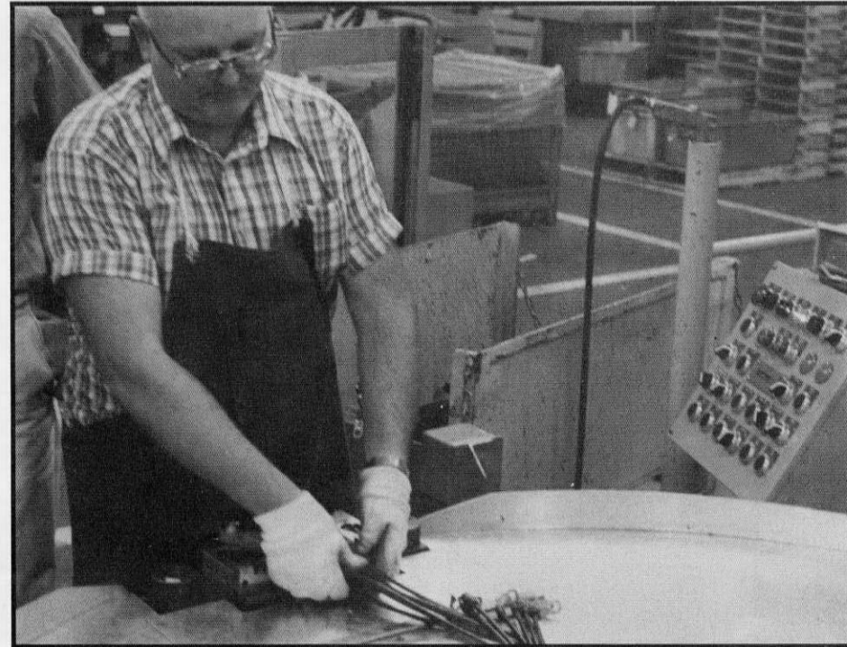
Jim Cosier, Dept. 1552, operates one of the two new rotary mold machines for the battery line.
