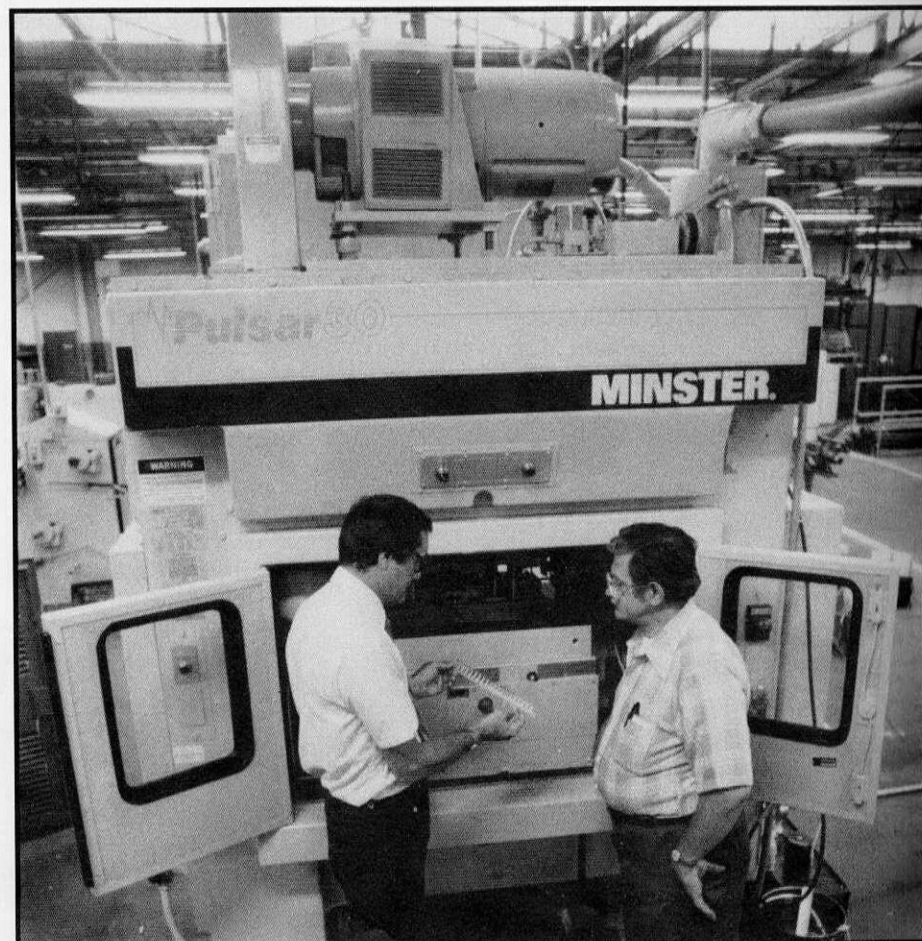
Mike Connolly, general foreman, and Norbet Bogdon, Dept. 1146, discuss the closed loop shut height system for a new Pulsar 30-ton Minster.
