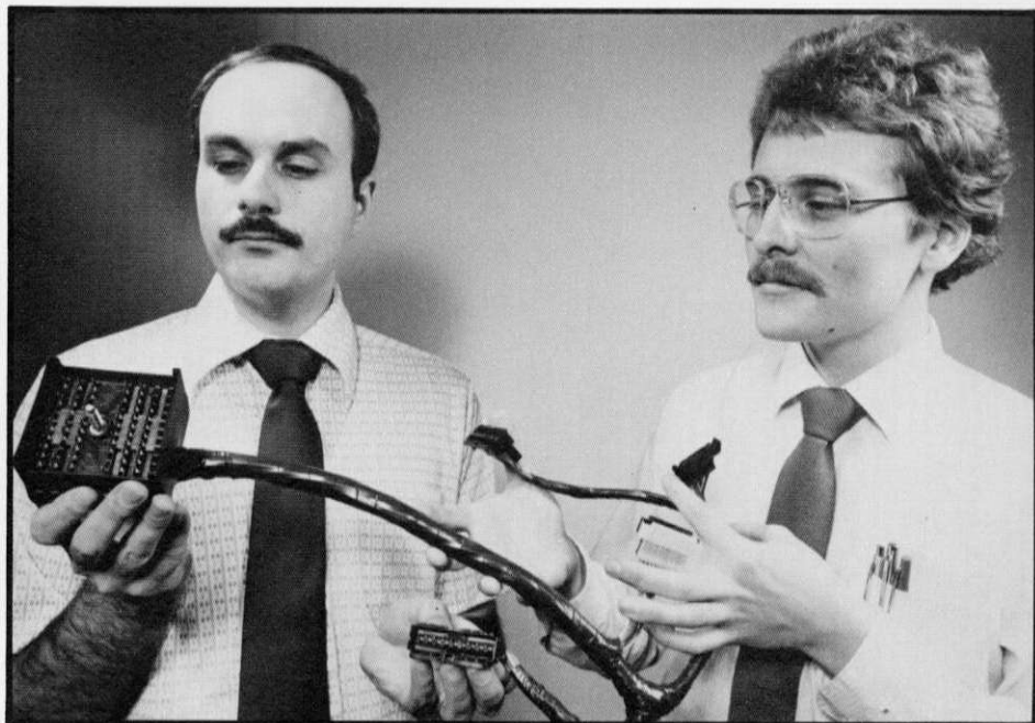
POSITIVE ROUTING CHANNEL (above) and pod wiring assembly (right) will be supplied by Packard Electric for GM's 1985 N car. Nick Pappoda (right), electrical engineer, and Mark Heacox (far right) mechanical engineer, hold pod wiring assembly.
