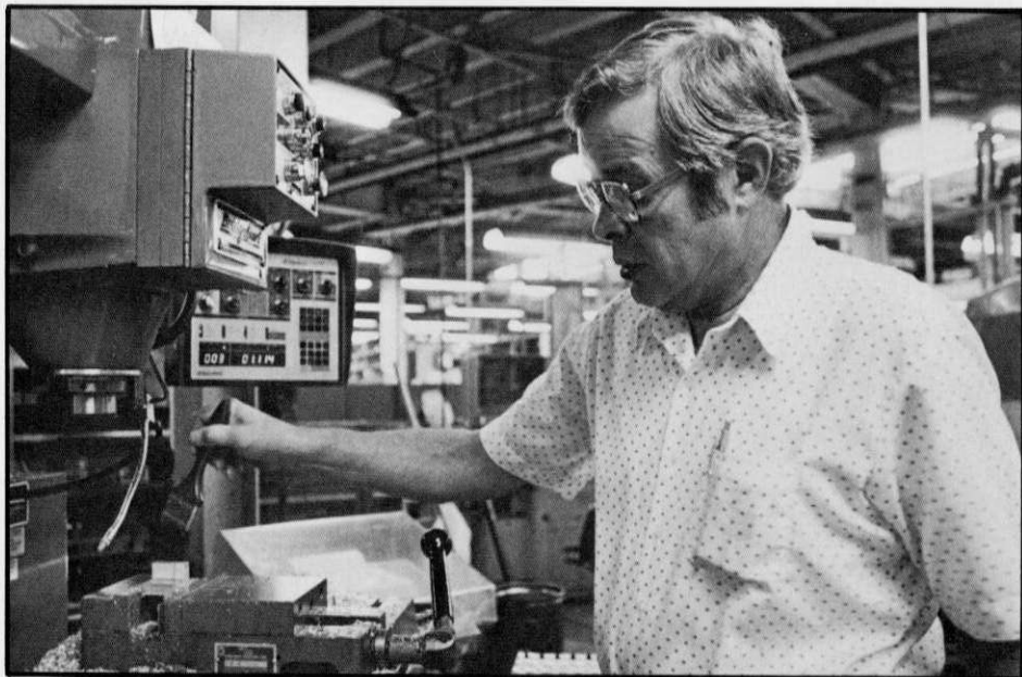
MILLING AROUND — machinist Bill Knappenberger, of Dept. 511, uses one of five numerically controlled milling machines in the shop to produce a Weather Pack connection tester.
