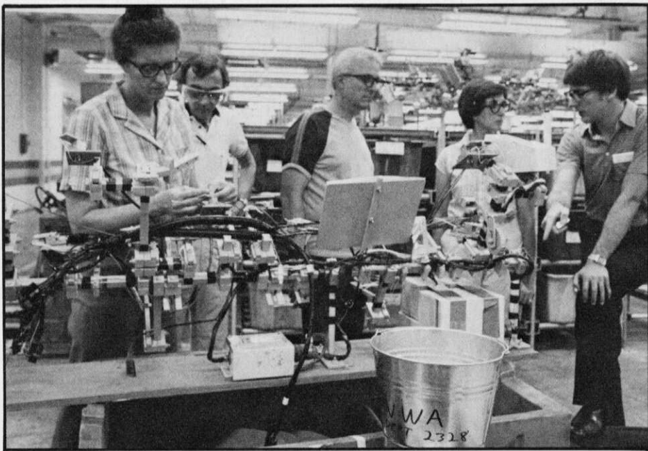
PACKARD EMPLOYEES from Warren and Brookhaven make the final check on a stationary board used for the Volkswagen engine harness being produced in Plant 23. The Volkswagen business is new for Packard and the production area will include 12 stationary boards, four part numbers and 17 employees in full operation. The first harness was produced July 22. Shown checking the board are, from left, Lyn Esparza, Nick Goodman, Albert Frederick, Dixie Moak and Larry Matola.
