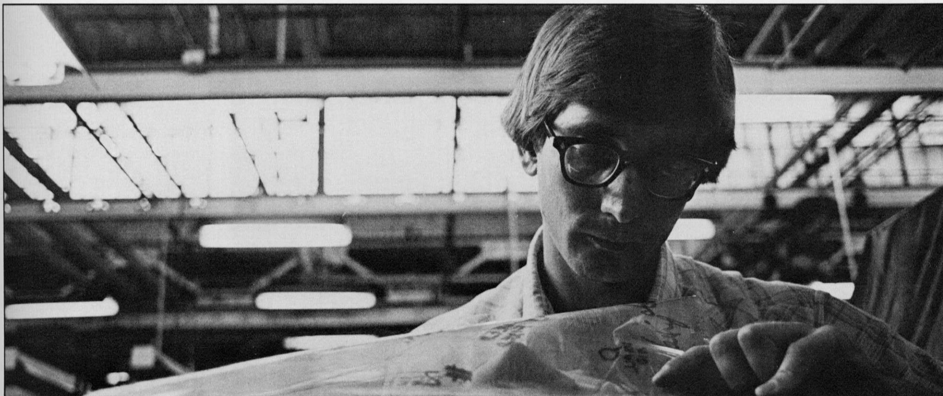
HIGHS AND LOWS — Tool and die maker Bruce Durst, Dept. 552, inspects a revised printed circuit die for high and low spots.
