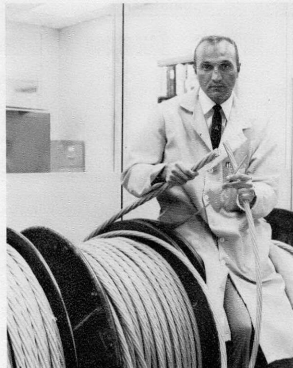
GLASTRAN is being produced in sizes from 1/16 to 1 inch in diameter. Anthony Bartholomew, Plastics Laboratory, shows some of the different sizes.
