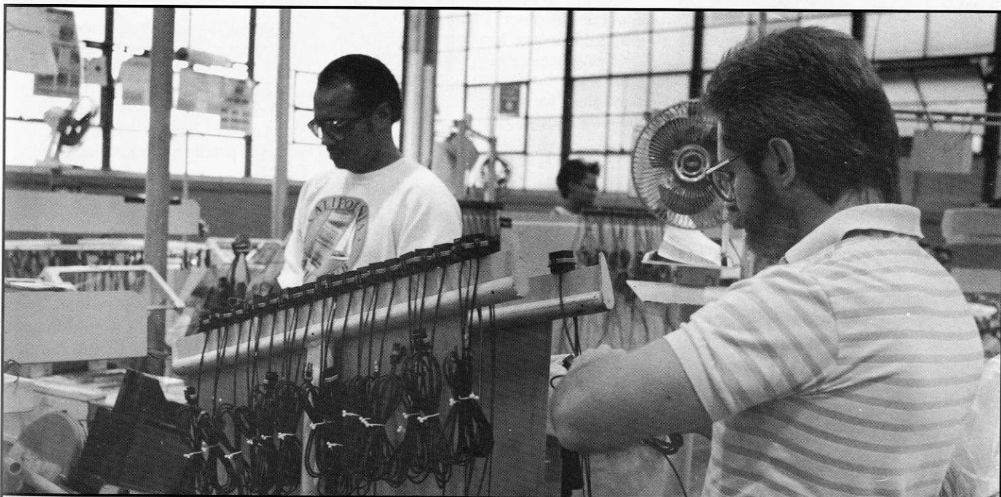
John Golias (right) coils pull-to-seat assemblies for buildability and material respect in Dept. 4907. This operation begins the synchronous process. Jim Crawley (left) then splices together pull-to-seat and cut lead assemblies. In effect, Golias' "dispose" become Crawley's "get."
