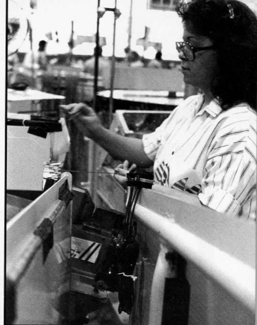
Paula Hoffman, Dept. 4907, splices together pull-to-seat assemblies and cut leads for coolant fan wiring harness sub-assemblies. This operation follows the coiling operation.
