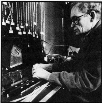
On the cover: John Gilliam, Dept. 808, checks a fiber optic ribbon to assure proper cutting. This product is used on GMC truck dashboard consoles.
