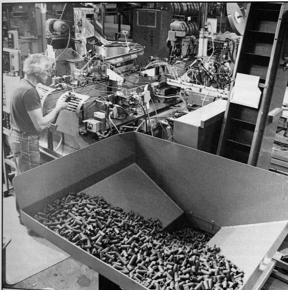
Jim Gray, Dept. 351, operates a High Energy Ignition (HEI) cutter with a double boot application. He checks the position of the boot on the terminal.
