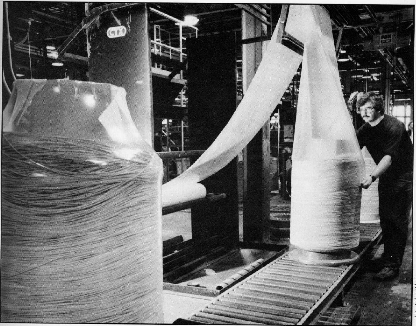
John Gray, Dept. 1045, service, covers a barrelless pack of wire with shrink wrap. Only the plastic base is returned to Packard after use by the customer.
