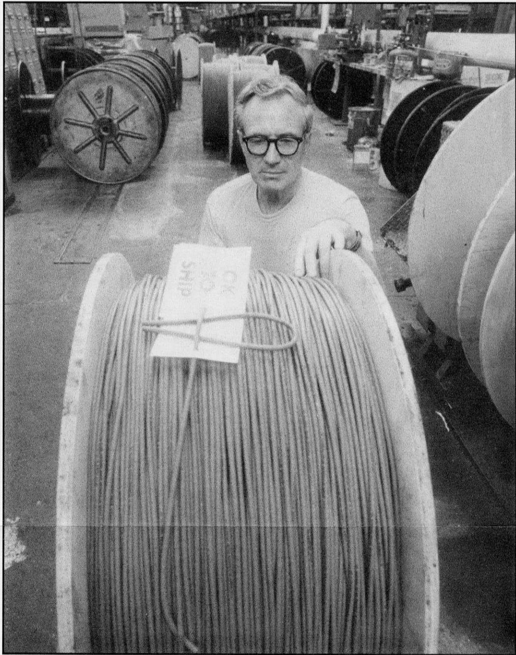
Watt Brown , CV operator, Dept. 322, prepares a reel of bulk ignition cable for shipment to the customer.
