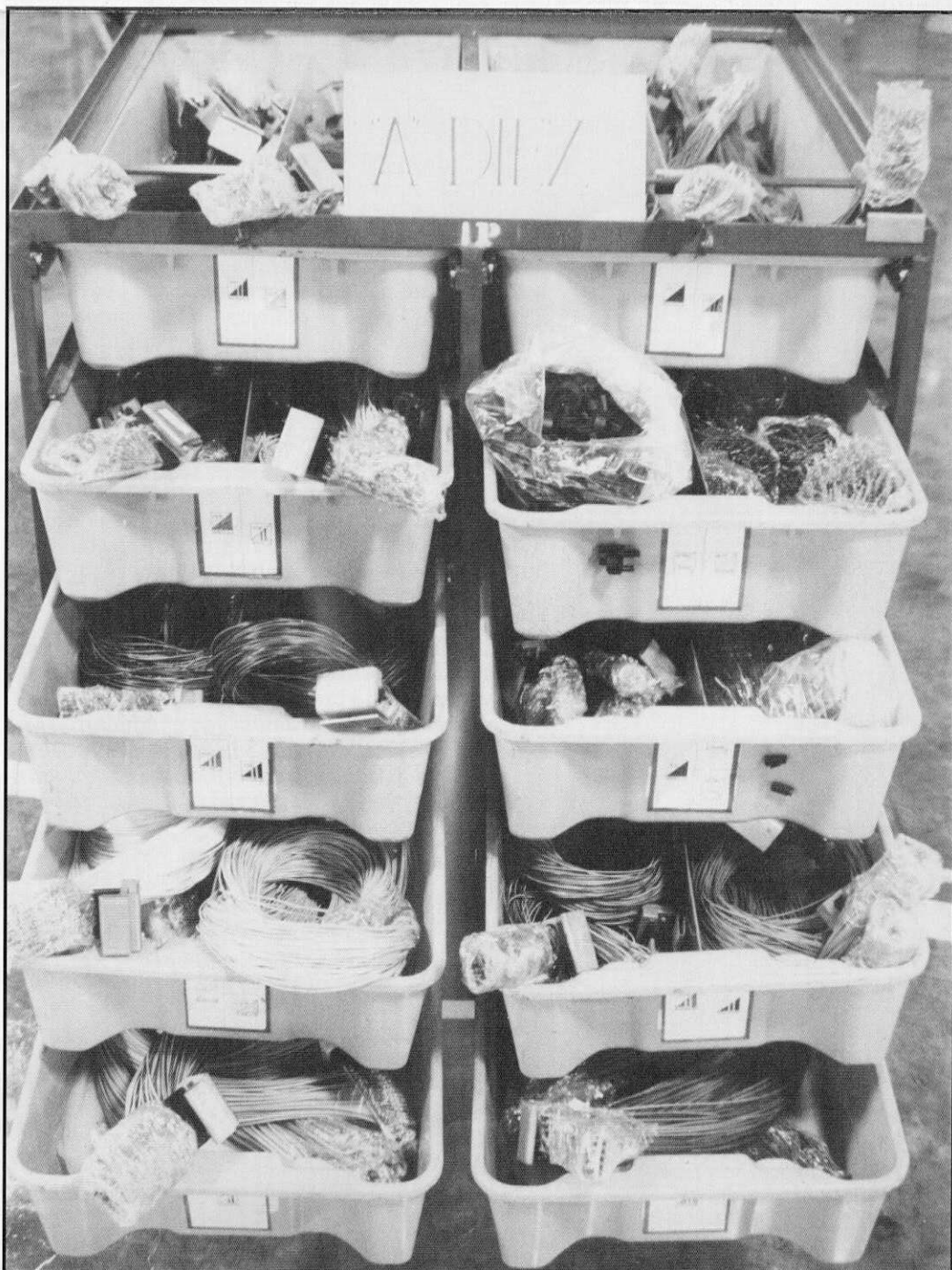
The Diez is a movable container made of 10 padded half cells which protect wire components while they are transported to the supplier. The Diez is one part of Mississippi's drive toward excellence.
