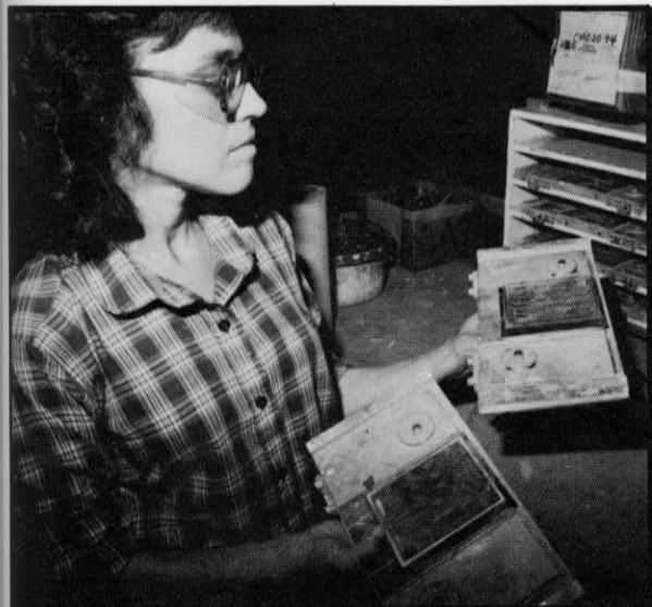
Mary Jackson, production operator in Dept. 2222, holds rubber pads used to imprint fuseblocks. At right is Clinton's transfer printer which can color code parts in six colors.
