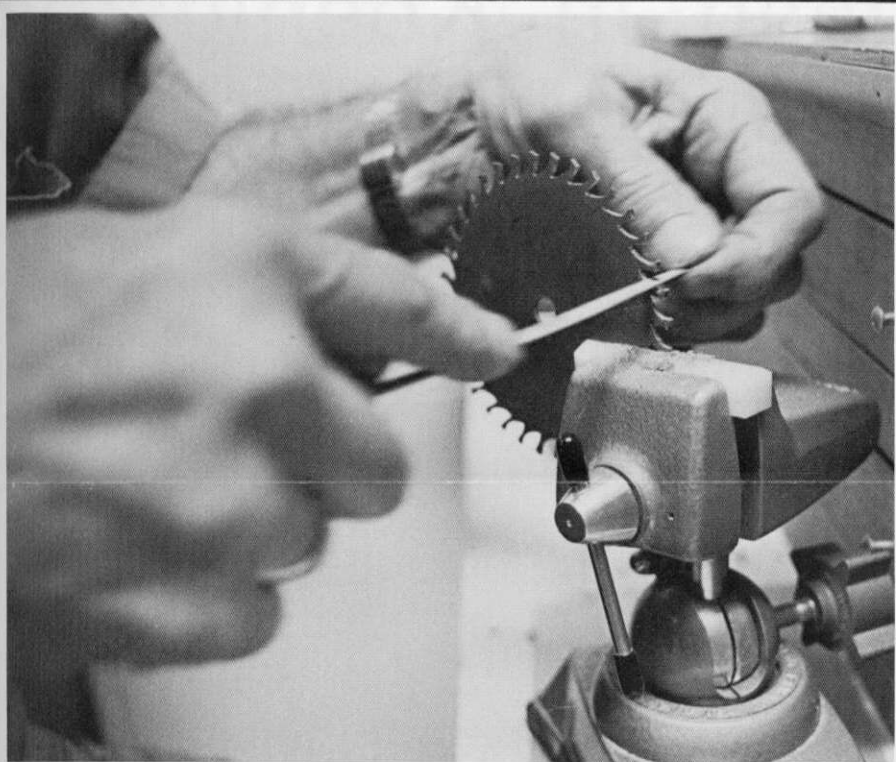
THE HANDS of Virgil Linger at work filing an escape wheel for one of his handmade clocks. More photos and a feature story appear on page three.
